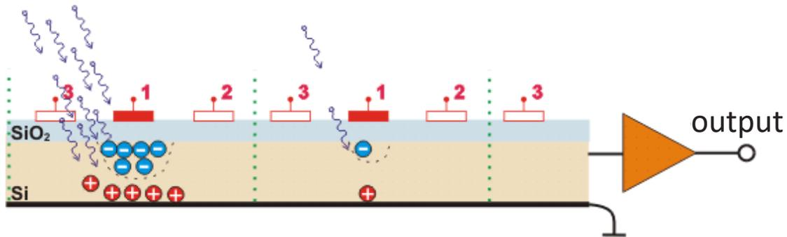
**Read-out:** altering potentials on electrodes charges are moved to output
