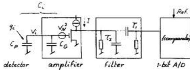
Fig. 1. Schematic drawing of the analog front end
