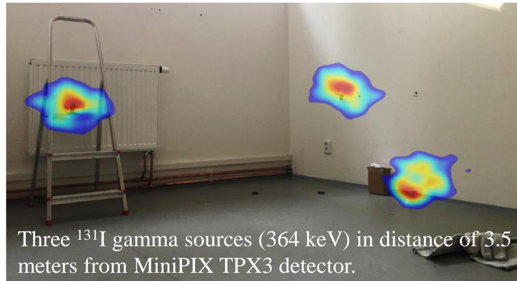
Three  $^{131}\text{I}$  gamma sources (364 keV) in distance of 3.5 meters from MiniPIX TPX3 detector.
